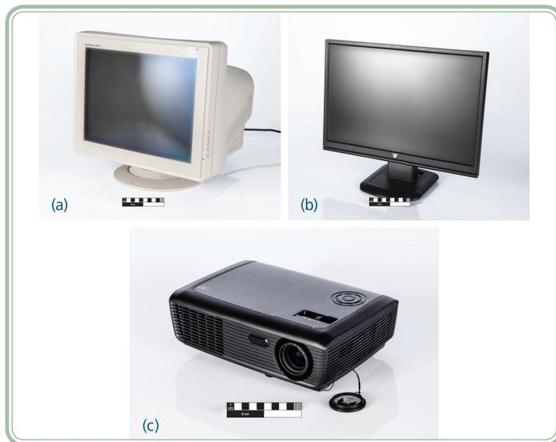
**Figura 2.12: Monitor CRT (a), monitor LCD (b) e projetor (c)**
