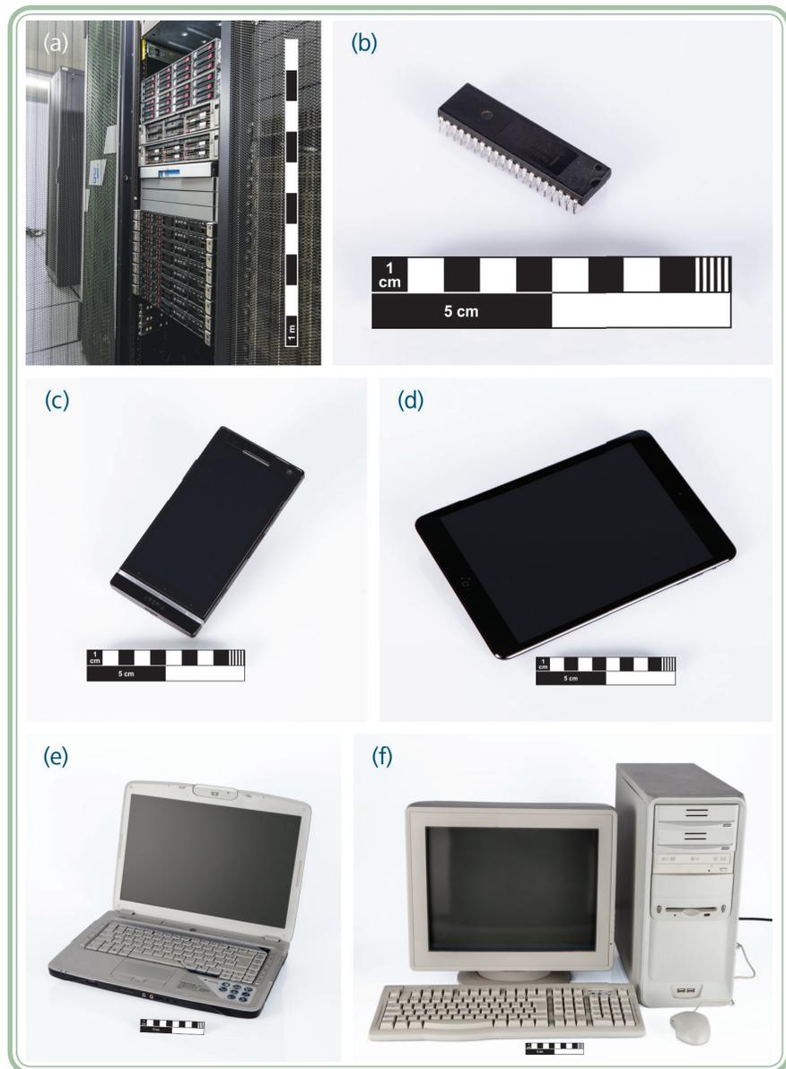
**Figura 1.2: Exemplos de computadores – mainframe (a), micro controlador (b), smart-phone (c), tablet (d), notebook (e), desktop (f)**
